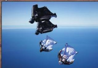
A new blended profile in the arm wing mixes standard camber and symmetric profile ribs across the span for improved backflying performance and overall agility.
